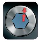
Hexagon socket screws can be problematic because of the very narrow contact surfaces that transfer torque from the tool to the screw. This can destroy the head of the screw. Hex-Plus tools provide a greater contact surface to prevent this and fit every standard hexagon socket screw.
